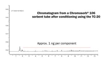
Although the precise conditions of temperature, carrier gas flow and time will vary depending on the nature of the work and the particular sorbent used, tubes should usually be conditioned for at least as long as their standard desorption time, using (where possible) higher temperatures and gas flows. Freshly packed tubes should be conditioned for much longer than this – typically at least 2 hours.
