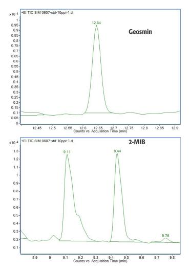
Fig 7: GC-MS chromatograms of Geosmin (top) and 2-MIB (bottom) at the regulated decision level 10 ng/L
