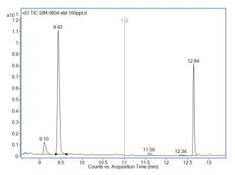
Fig 5: GC-MS chromatogram of 2-MIB and Geosmin aqueous solution (100 ng/L) by SPME Arrow extraction
