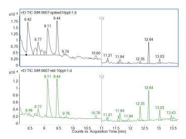
Fig 11: Water sample chromatograms, spiked at 10 ng/L (above, the spiked drinking water sample, below a spiked ultra-pure water preparation)
