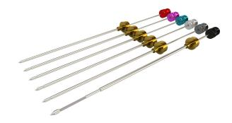
Fig 4: Color coded SPME ARROW devices
