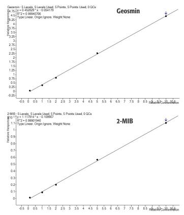
Fig 6: Calibration curves of Geosmin (top) and 2-MIB (bottom), both in the range of 1 to 100 ng/L with precision better than R2=0.999
