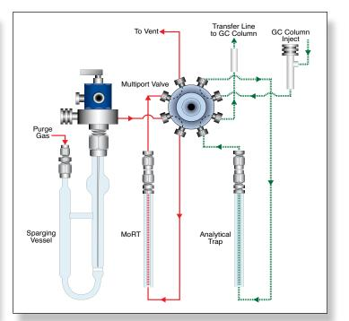
Desorb – 8-port valve separates the desorb flow from the GC away from the moisture control, decreasing the sample path length between the trap and GC
