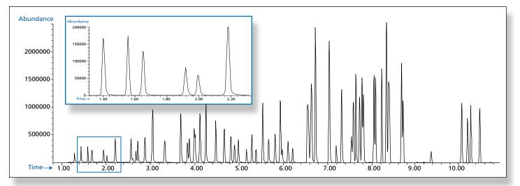
50 ppb EPA Method 8260 on a 6890/5973 GCMS. Front end gases showing improved resolution are highlighted.
