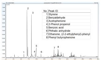
Figure 1. Photo-thermal oxidative degradation products of polystyrene
