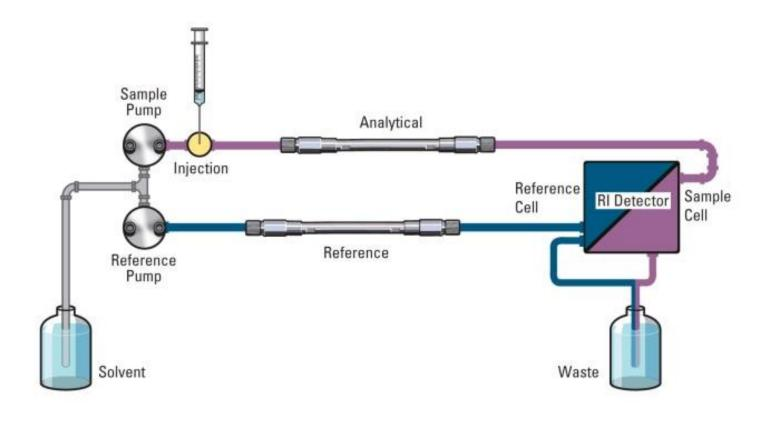
Dual flow RI detector results in low noise and baseline drive, maximum sensitivity, rock steady baselines, and fast system equilibration
