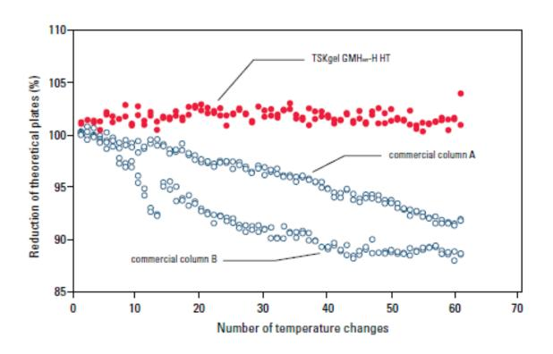
TSKgel GMHHR-H HT column showed stable performance during repetitive rise and fall of column temperatures up to 60 cycles.
