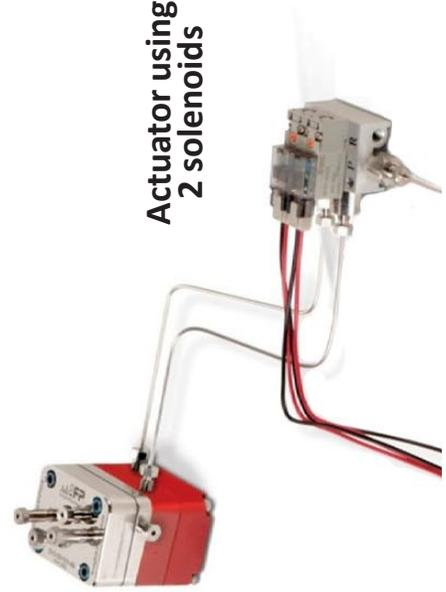
**Actuator using 2 solenoids**
